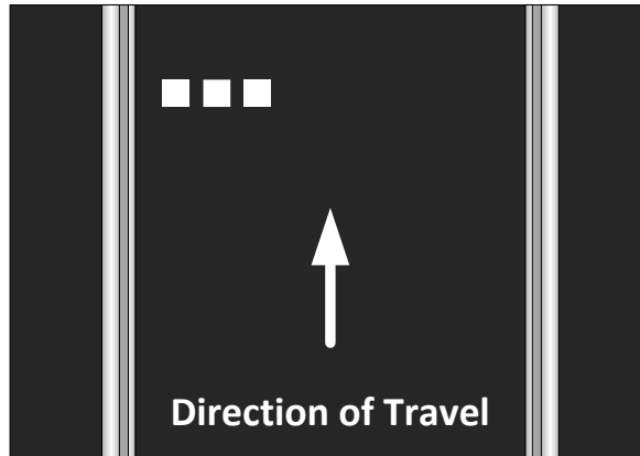
Figure 19 - Stopping Place Studs
