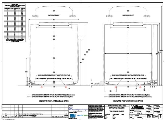
Figure 2 - Kinematic Outline (Dimensions are in mm)
